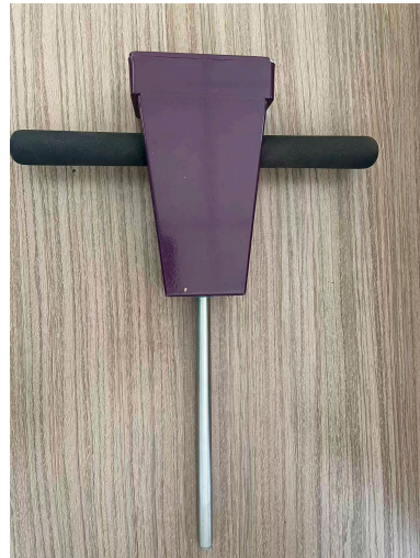
Figure 1. SC900 soil compactness meter.
