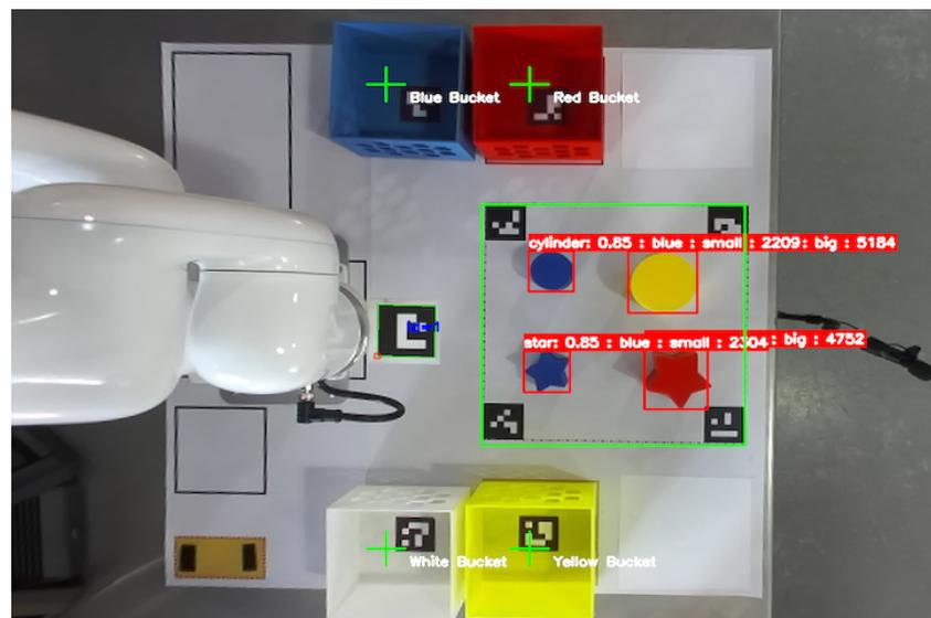
Figure 5. Top view of the working area with objects detected using YOLOv8N.
