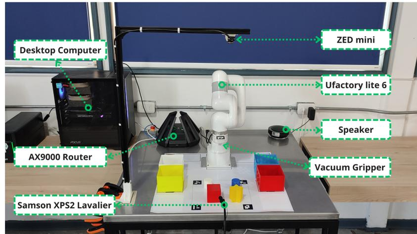
**Figure 1.** Detailed view of the experimental setup, showcasing its various components.
