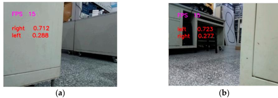
**Figure 10.** Scene recognition, distinguish left turn or right turn where (a) 15 frames per second, the score for left turn is 0.288 and the score for right turn is 0.712 (therefore, it is judged as right turn) and (b) 15 frames per second, the score for left turn is 0.723 and the score for right turn is 0.277 (therefore, it is judged as left turn).
