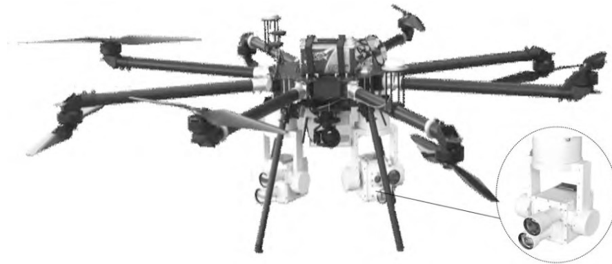
Figure 5. Physical image of unmanned aerial vehicle's laser communication equipment.
