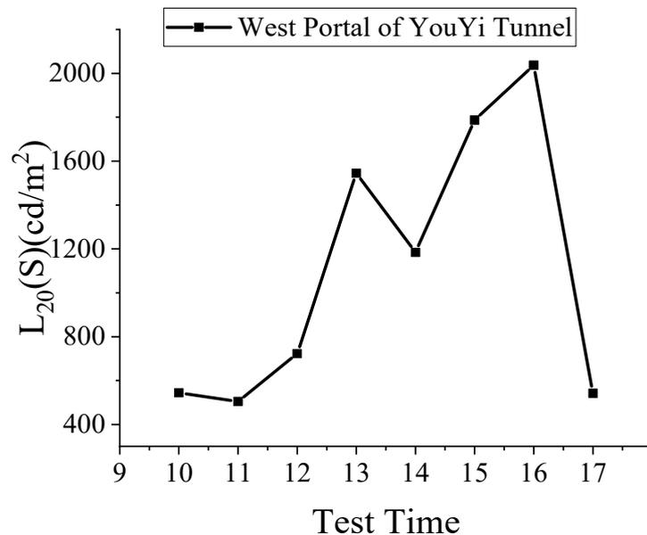
Figure 5. Measured  $L_{20}(S)$  value at the west portal of Youyi Tunnel.
