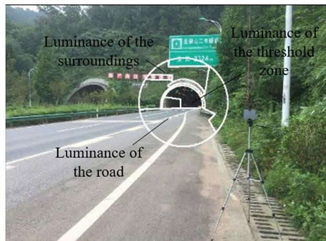
**Figure 2.** Test block diagram of Longquanshan No. 2 Tunnel.
