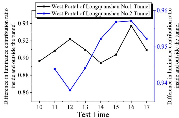
**Figure 12.** Difference in luminance contribution ratio of the west oriented tunnel. (Longquanshan No. 1 Tunnel, Longquanshan No. 2 Tunnel).
