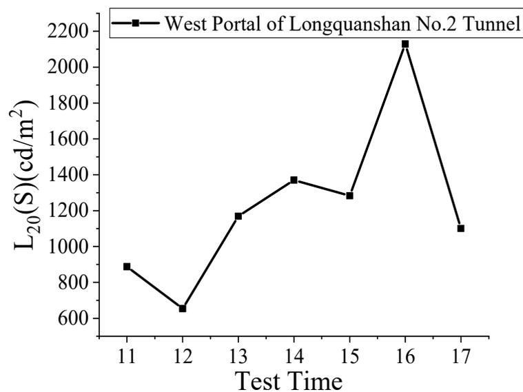
**Figure 7.** Measured  $L_{20}(S)$  value at the west portal of Longquanshan No. 2 Tunnel.
