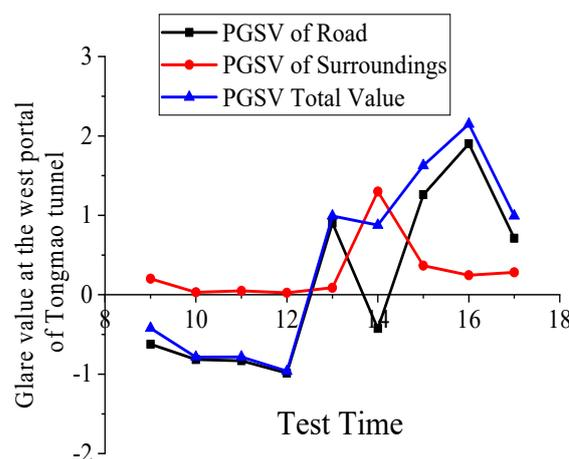
Figure 17. PGSV for the west portal of the Tongmao Tunnel.
