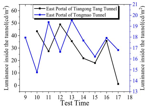
Figure 9. Luminance inside the due east oriented tunnel.
