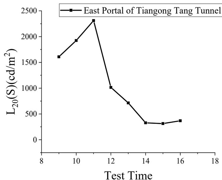
**Figure 3.** Measured  $L_{20}(S)$  value at the east portal of Tiangongtang Tunnel (Summer).
