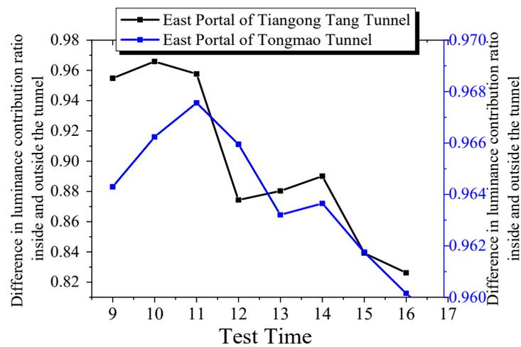
Figure 11. Difference in luminance contribution ratio of the east oriented tunnel.
