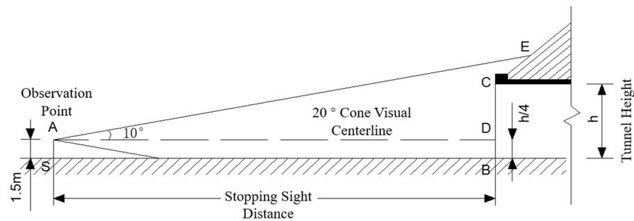
**Figure 1.** Schematic of  $L_{20}(S)$  test.
