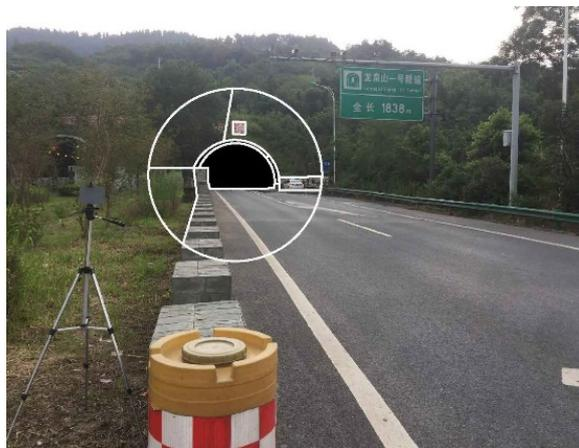
Figure 14. Road tunnel light and dark background block diagram.
