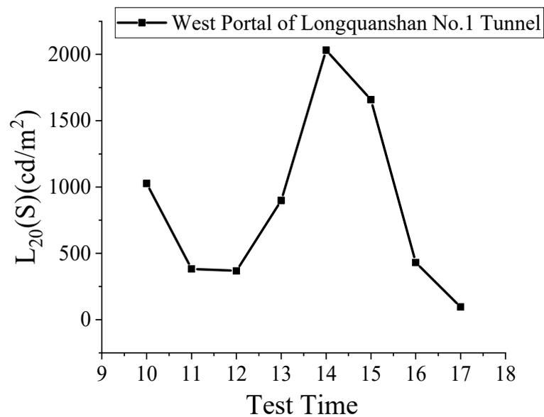
**Figure 6.** Measured  $L_{20}(S)$  value at the west portal of Longquanshan No. 1 Tunnel.
