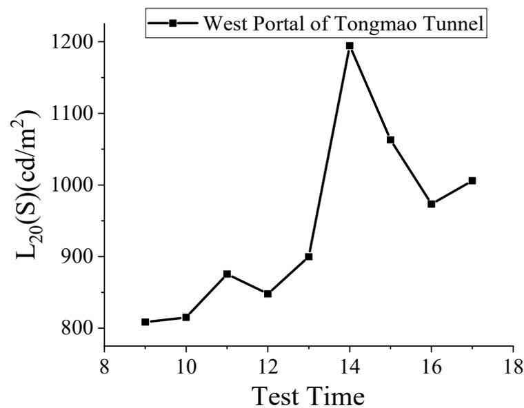
**Figure 8.** Measured  $L_{20}(S)$  value at the west portal of Tongmao Tunnel.
