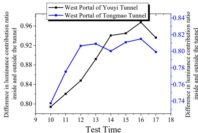
**Figure 13.** Difference in luminance contribution ratio of the west oriented tunnel. (Youyi Tunnel, Tongmao Tunnel).
