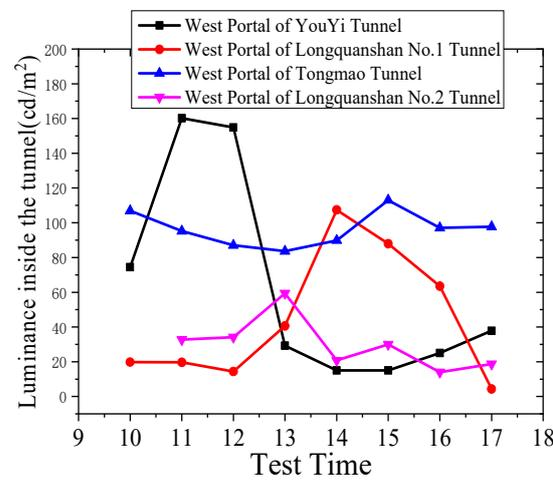
Figure 10. Luminance inside the due west oriented tunnel.
