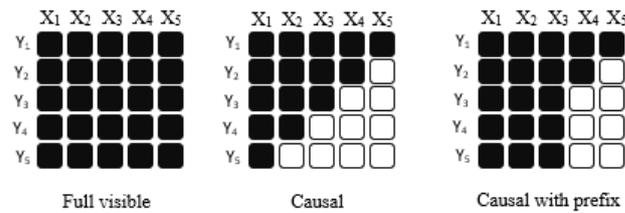
Figure 5. Different mask types in attention mechanism.
