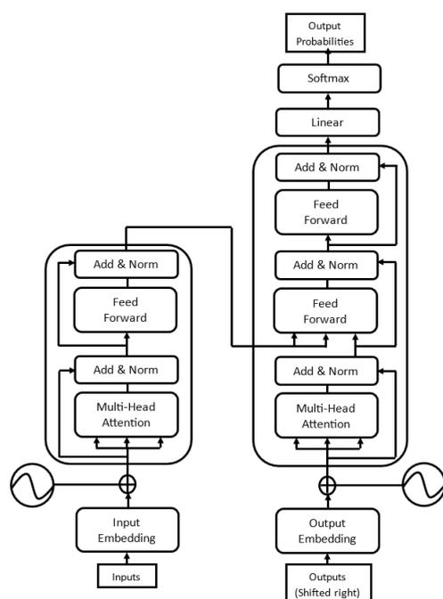
Figure 3. Transformer's encoder–decoder-based model.
