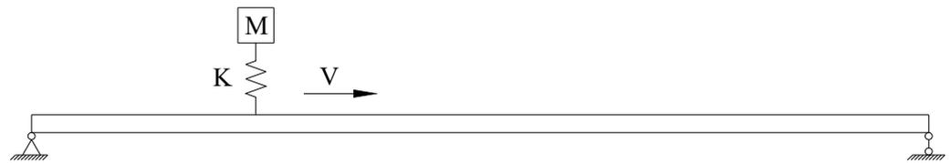
Figure 3. Uniform moving spring-mass system acting on a simply supported girder.
