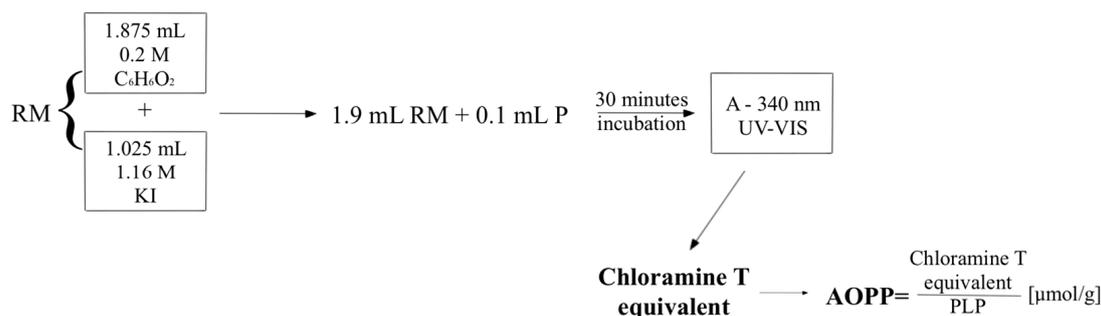
**Figure 1.** Method of determination of the advanced oxidation protein products concentration; A: Absorbance; RM: Reactant mixture; P: Plasma; PLP: protein level in plasma.
