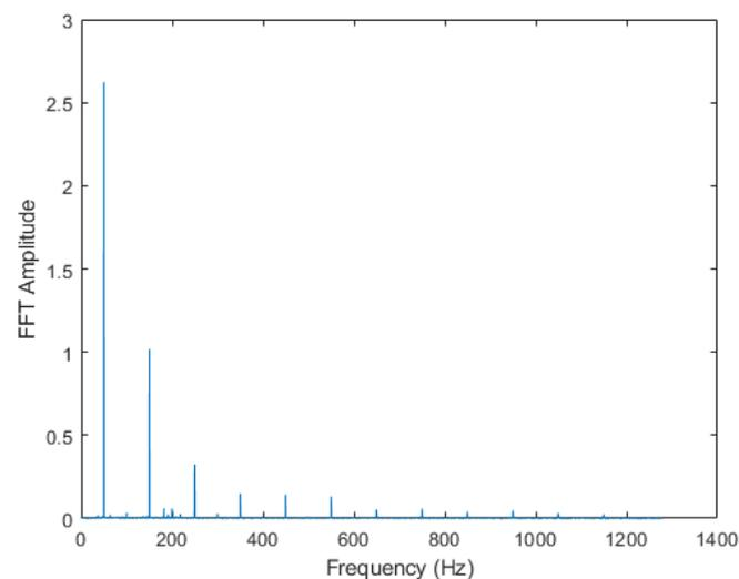
**Figure 4.** FFT spectrum of a signal vibration measured along the z-axis for a half-used belt.
