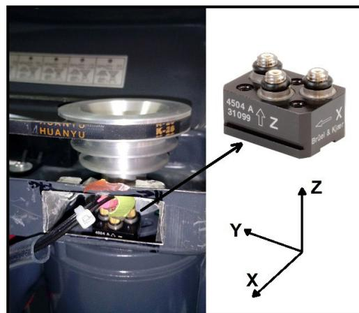
**Figure 1.** Final assembly of the triaxial accelerometer (Brüel & Kjaer 4504A).
