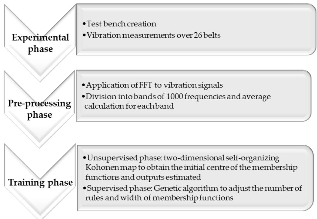
**Figure 5.** Flowchart of the process.
