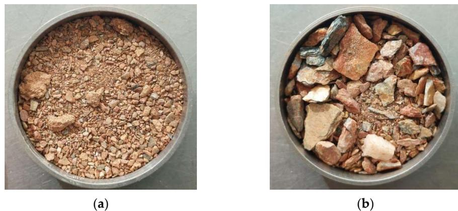
**Figure 2.** (a) Appearance of R1 soil (maximum particle size < 2 mm), and (b) appearance of R2 soil (maximum particle size < 12.5 mm).
