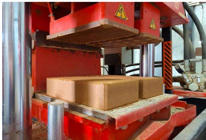
**Figure 3.** Freshly compressed earth blocks (R1 type).
