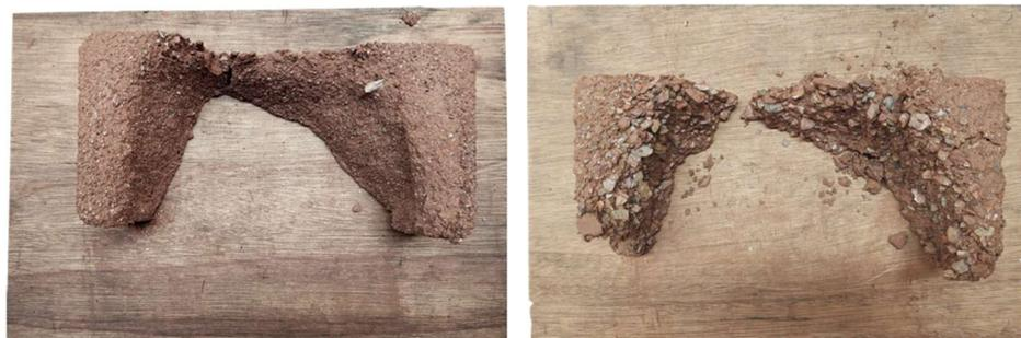
Figure 14. Condition of the blocks after spray erosion test.
