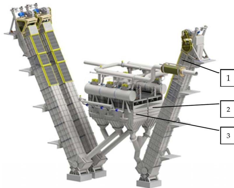
**Figure 2.** Jig node: 1—bucket conveyor, 2—jig 1 (3 compartments), 3—jig 2 (3 compartments).
