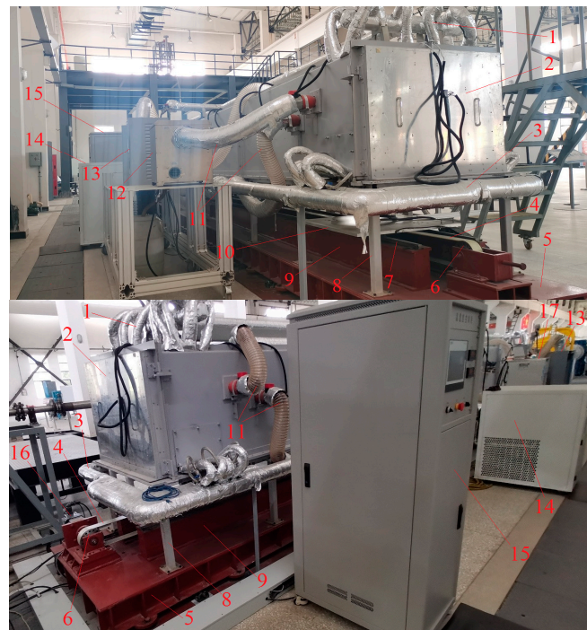
Figure 3. The assembly of the mechanical structure system. 1. Water intake pipes; 2. Enclosed chamber; 3. Water return pipes; 4. Synchronous belt; 5. Mounting platform; 6. Synchronous pulley; 7. Guide track; 8. Chamber propping pillars; 9. Guide track pedestal; 10. Moving flat plate carriage; 11. Steam (moist air) pipes; 12. Recirculating dehumidifier; 13. Humidifier; 14. Constant-temperature water tank; 15. Temperature and humidity control cabinet; 16. Driving motor; 17. Recirculating heating/refrigerating machine.
