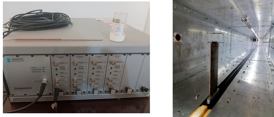
Figure 17. The hot-wire anemometer, its probe, and the probe fixed on the strut in the enclosed chamber.
