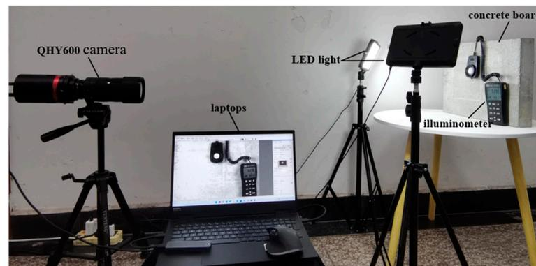
Figure 3. Arrangement of the experimental devices.
