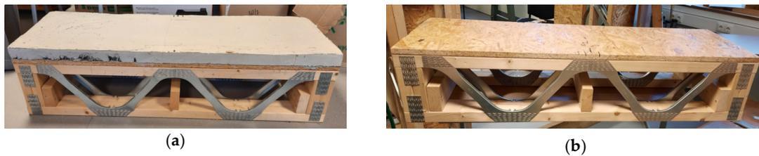
**Figure 1.** Considered specimens with posi-joisted beams: (a) with a concrete layer; (b) without a concrete layer.
