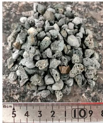
**Figure 1.** Appearance of expanded shale LWAs.
