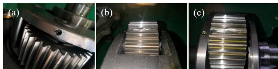
**Figure 11.** Faulty gear condition. (a) Minor tooth failure state. (b) Moderate tooth failure state. (c) Severe tooth failure state.
