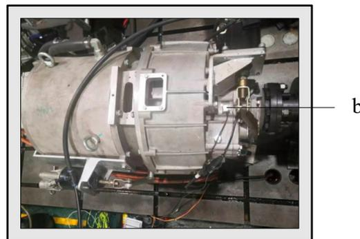
**Figure 10.** The mounting position of the accelerometer.
