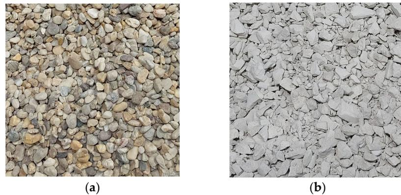
**Figure 1.** Aggregates: (a) Quartz gravel; (b) RA of 3D-printed concrete waste.
