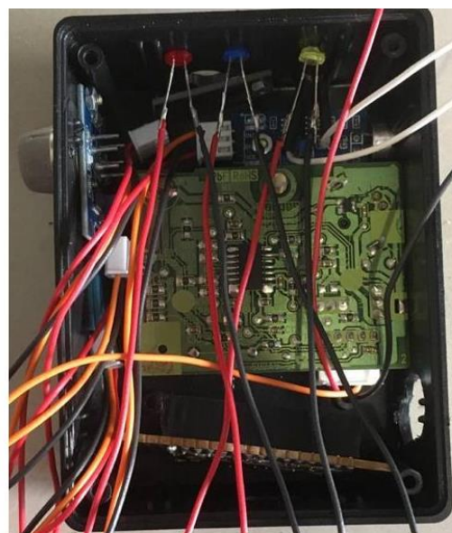
Figure 2. ESP32 and sensors (a) and device assembled (b).
