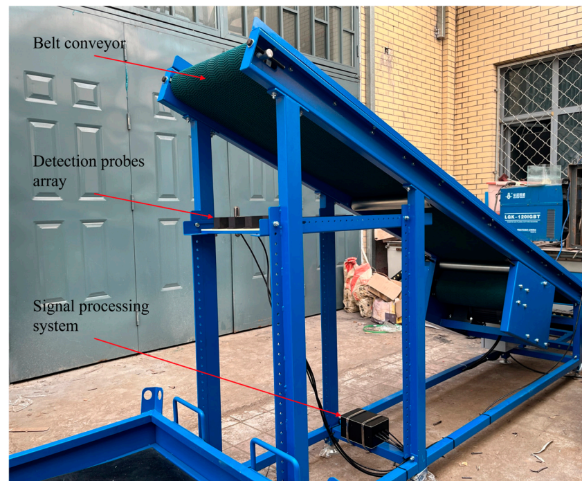
Figure 12. Field experiment platform with the multi-probe array.
