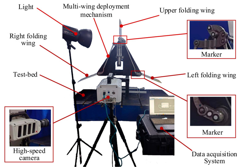
Figure 17. Experimental test of multi-wing deployment mechanism.
