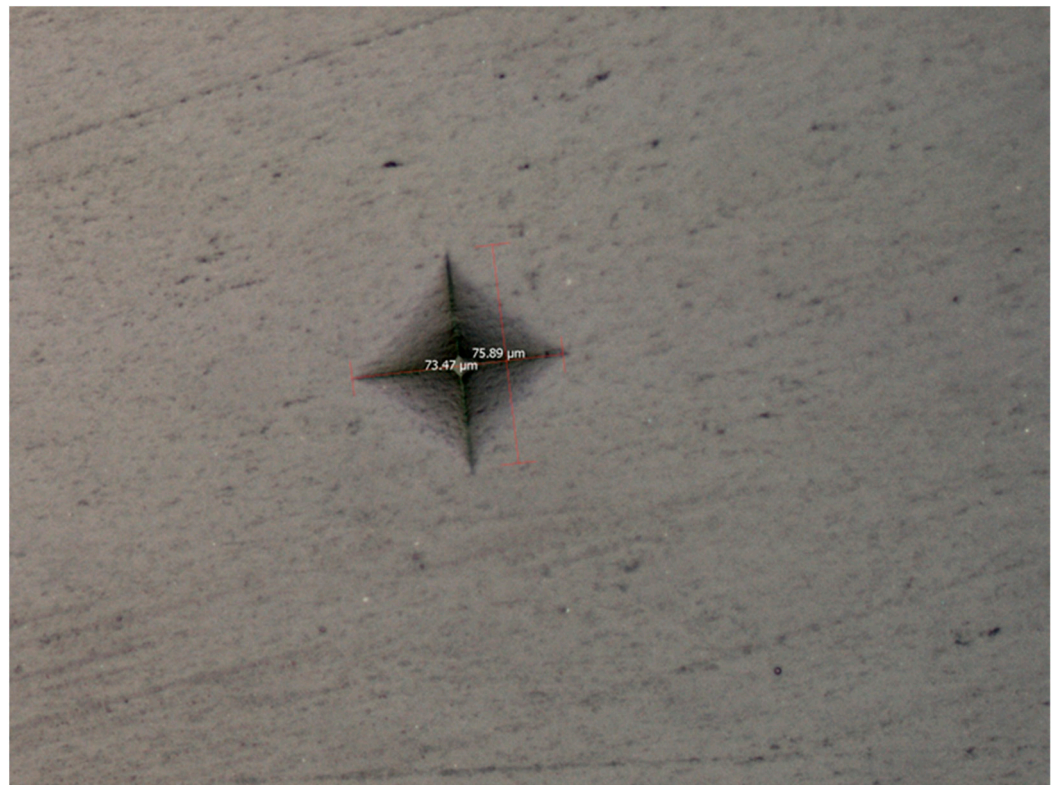
Figure 4. The Vickers microhardness indentation and the dimensions of the diagonals of a Tetric Evo Ceram Bulk Fill specimen polymerized by the Elipar LCU at a depth of 2 mm.
