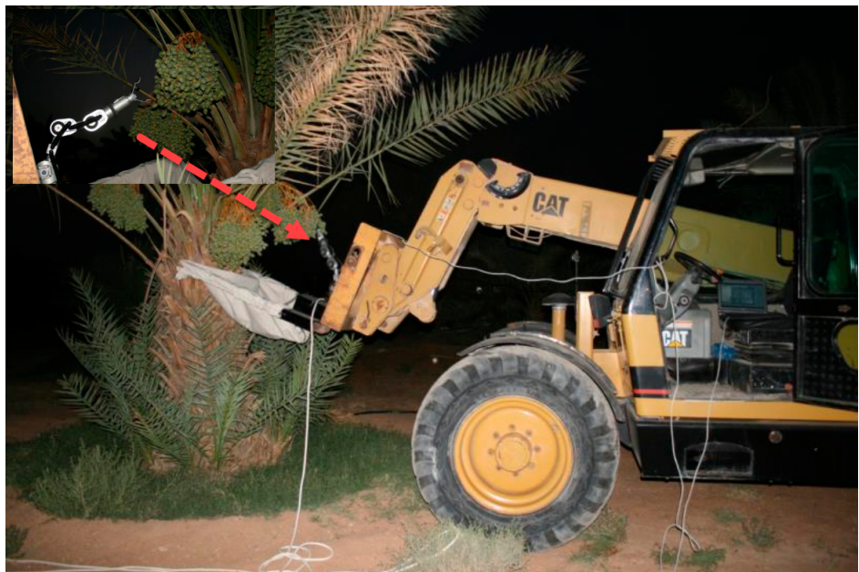
Figure 3. Robotic arm for date harvesting [16].
