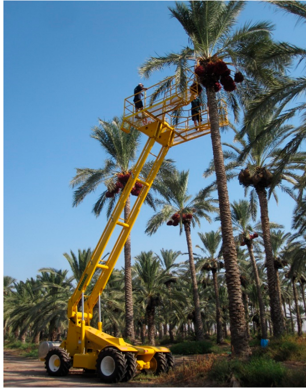
Figure 2. Hydraulic lift for palm tree harvesting.
