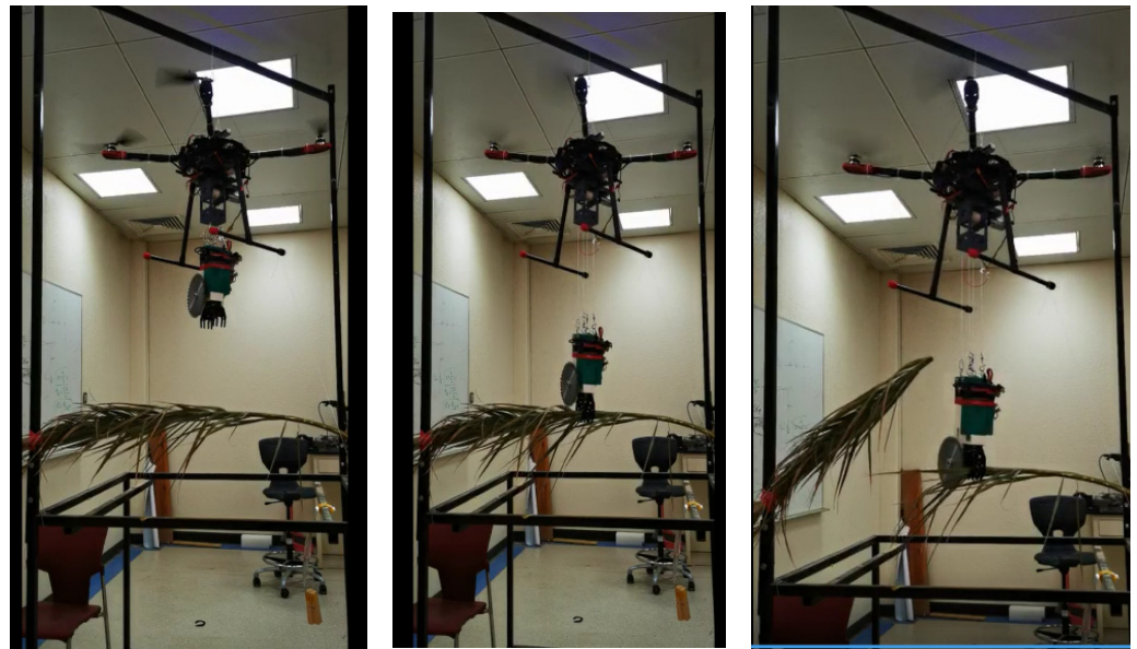
Before operating the winch After operating the winch After completing the cutting
