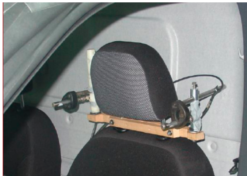
Figure 1. Position of microphones in drivers' seat.
