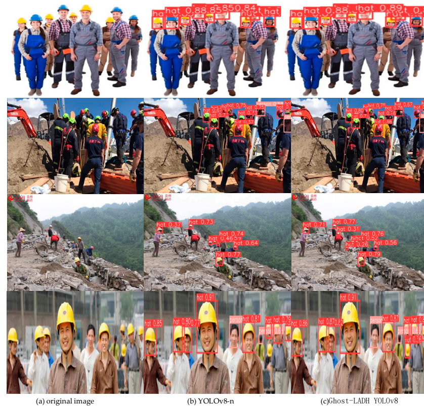
Figure 12. Visualization results for different scenarios (adapted from ref. [35]). (a) The pictures in the original dataset and the helmet detection pictures in different scenarios; (b) Base model YOLOv8-n; (c) Improved model LG-YOLOv8.
