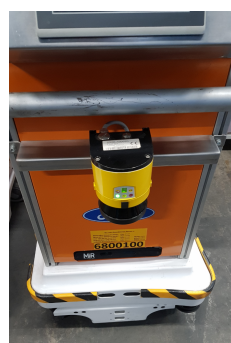
Figure 4. Additional sensor to avoid collisions with objects in different positions.
