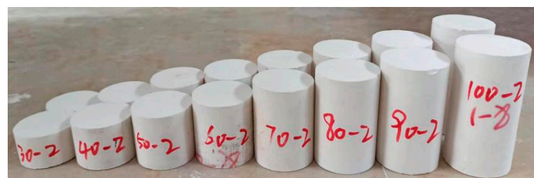
Figure 3. Part of the specimens with different HDRs.
