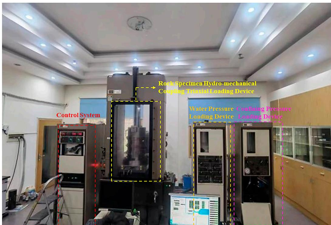
Figure 1. Rock triaxial seepage test system.
