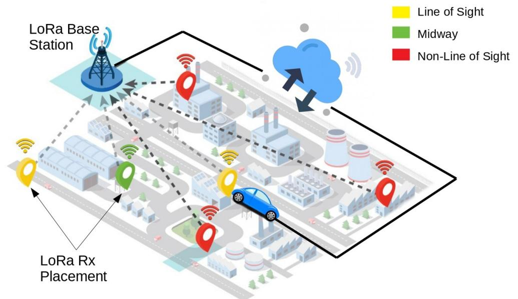
**Figure 1.** Testbed for the LoRa wireless sensor node deployment.
