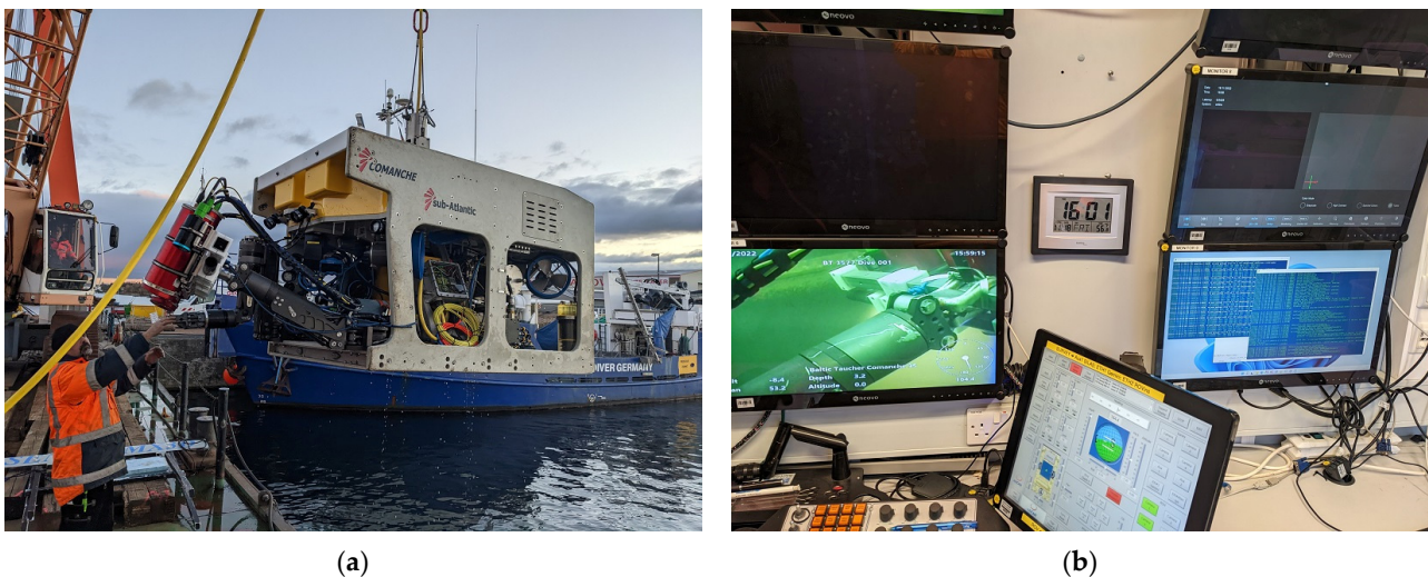
Figure 6. UWS mounted on ROV immediately before measurement application (a) and control room for UWS and ROV on the ship (b).
