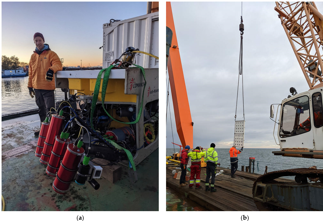
Figure 7. UWS mounted on ROV (a) and placement of the ArUco markerboards into the water (b).
