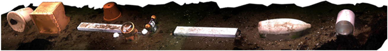
Figure 8. Reconstruction result of line of test objects using visual odometry and color mapping.
