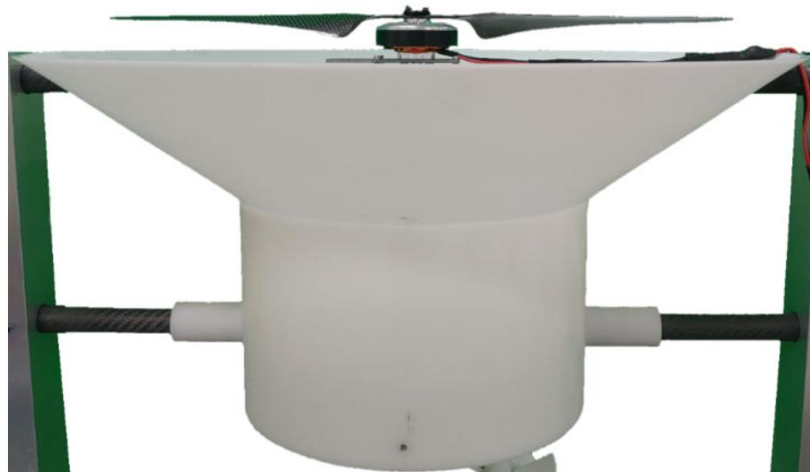
**Figure 14.** Wind collecting hood with a vertical flight rotor.
