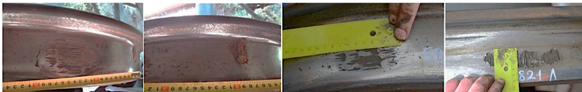
Figure 9. Wheel damage—flat and cracks [71].
