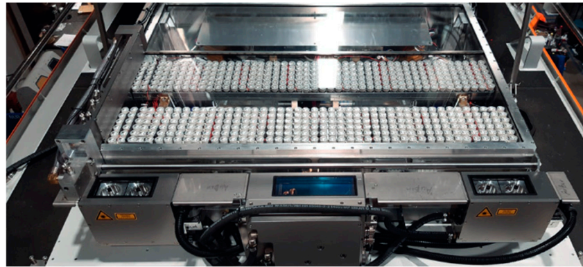
Figure 7. CIS with open lid showing the individual sensors: CRS (middle bottom), two LPS (left and right bottom), and LED panels for illumination. The cameras for wire-wear measurement are located between the LED panels (not visible). The metal rails are used for the semi-automatic cleaning system.
