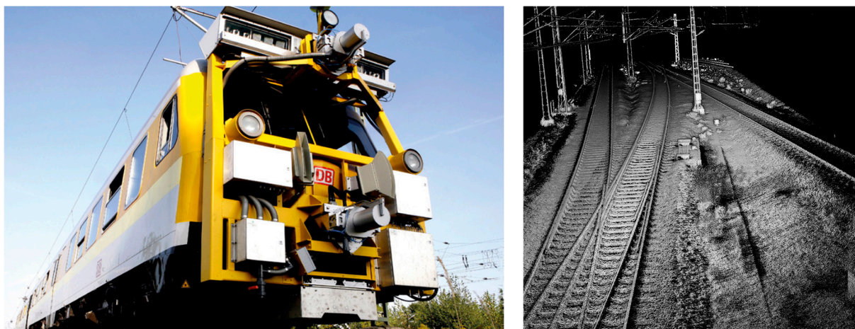
Figure 8. (Left) High-Speed Profiler (HSP) system from Fraunhofer IPM with two sensor heads mounted on the Deutsche Bahn inspection train LIMEZ III. (Right) Image of a point cloud captured by HSP.
