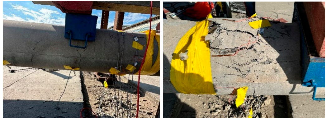
Figure 7. Cracking before and after failure of PCFRP1000.
