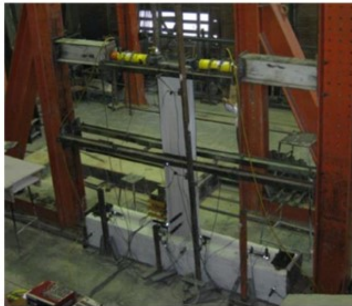
Figure 5. Full-scale test bench of the WUF-W connection with square section column.
