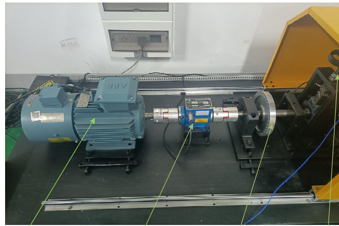
High-speed inverter motor Torque Speed Sensor Load balancing disk Radial loader
