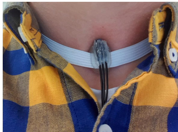
Figure 12. Placement of the sensor on the larynx using the 3D printed accelerometer support made of resin.
