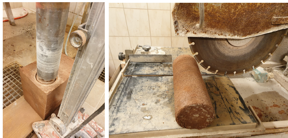
Figure 11. (Left) cutting a cylindrical specimen 100 mm in diameter from a rectangular block. (Right) trimming the specimen to a height of 100 mm [48].
