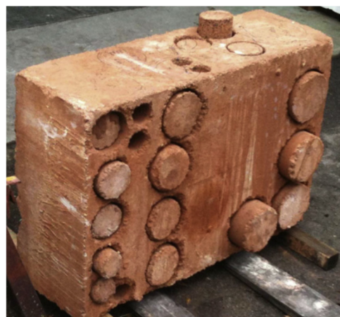
Figure 3. Coring specimens from the CSRE element. The specimens were cored both vertically and horizontally [11].
