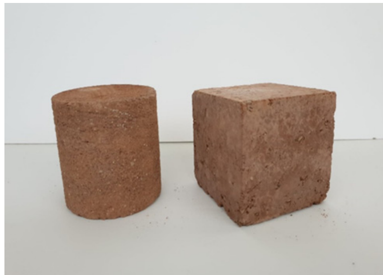
Figure 12. (Left) cored cylindrical specimen. (Right) cubic specimen.
