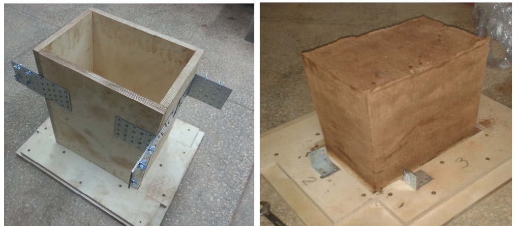
Figure 10. (Left) formwork for the specimen. (Right) specimen after forming.
