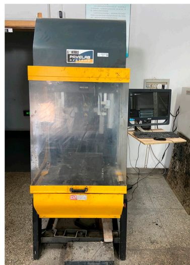
Figure 2. Controls pavement roller.
