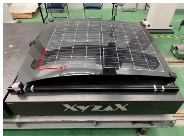
Figure 4. Coordinate measurement of the curved PV modules with the carrier.
