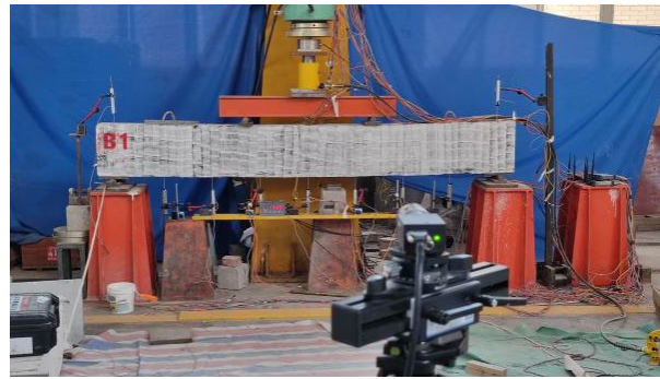
Figure 7. Test beam loading photo.
