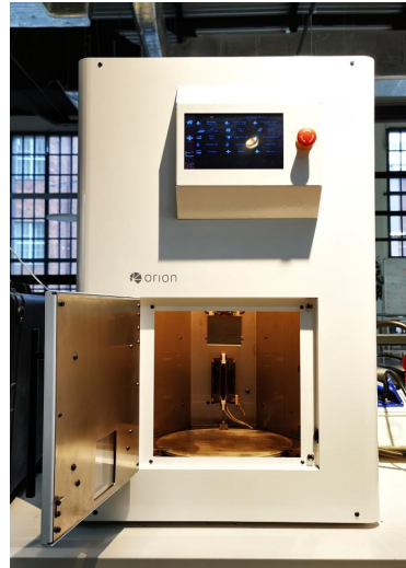
Figure 2. Orion's medical grade A150 3D printer, taken from [15]. Outer dimensions: 570 mm × 550 mm × 830 mm. Build volume: 180 mm diameter × 150 mm high.
