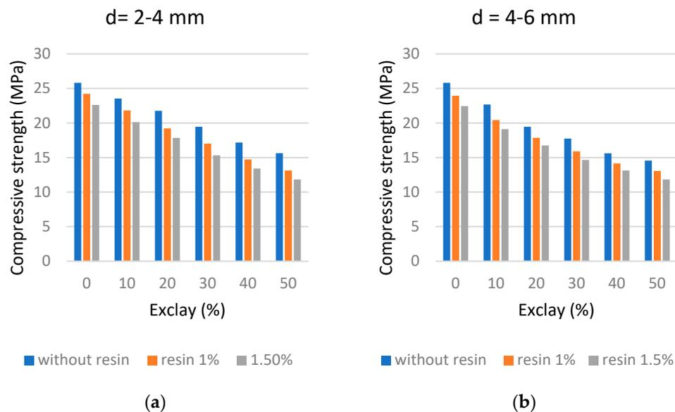
**Figure 7.** Compressive strength with respect to exclay ratios: (a) 2–4 mm, (b) 4–6 mm.
