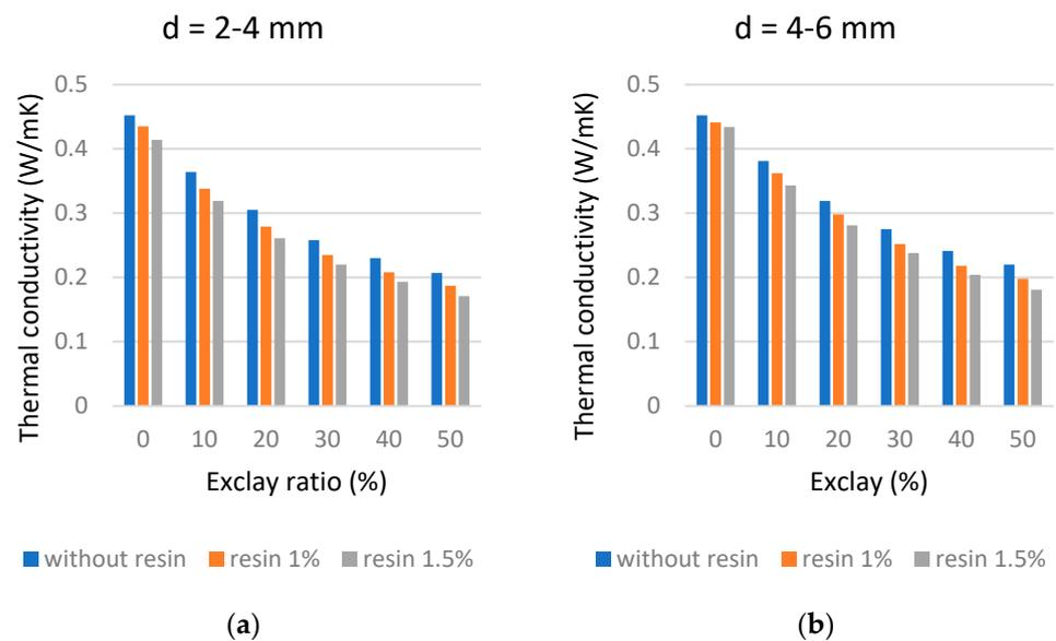
**Figure 6.** Thermal conductivities with respect to exclay ratios: (a) 2–4 mm, (b) 4–6 mm.
