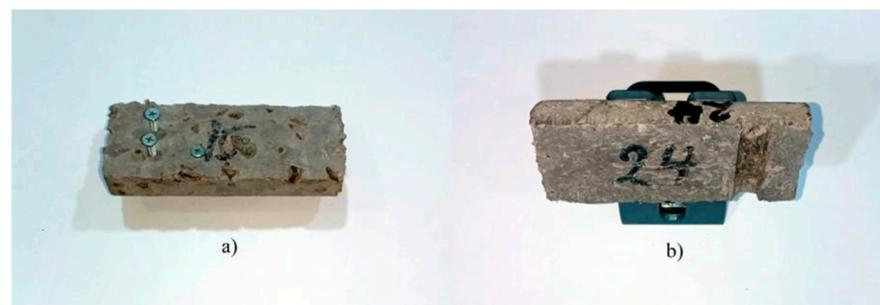
**Figure 10.** Mechanical applications on samples: (a) screwing and drilling, (b) grooving.
