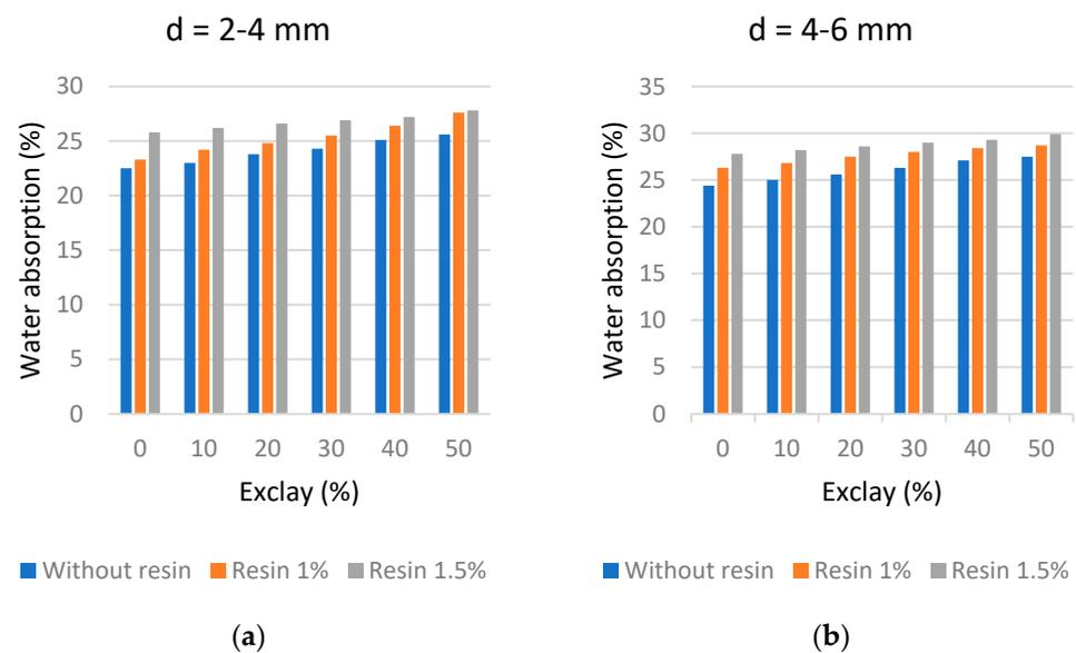
Figure 8. Water absorption ratio of samples versus exclay ratios: (a) 2–4 mm, (b) 4–6 mm.
