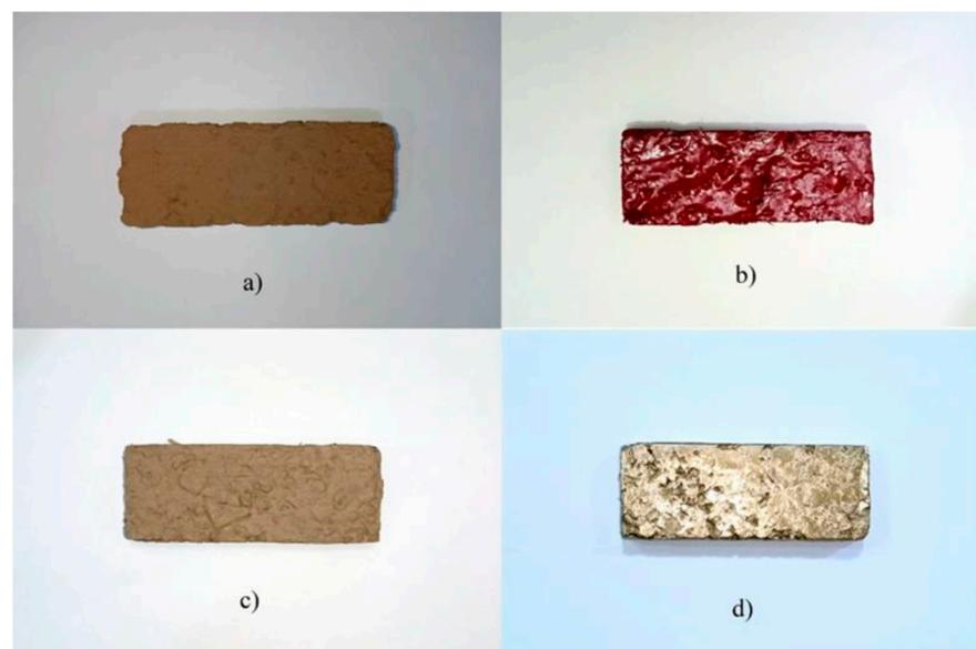
**Figure 9.** Painted samples. (a) Water-based silicone, (b) oil paint, (c) acrylic paint, (d) golden metallic paint.
