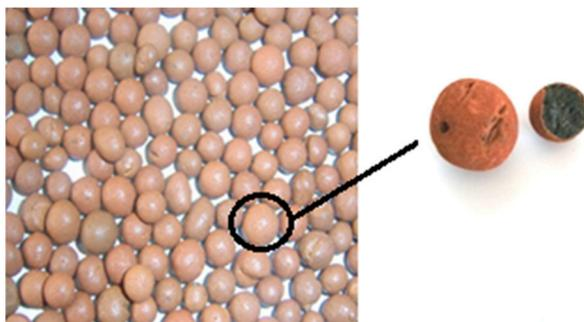
**Figure 1.** View of the exclay aggregate.
