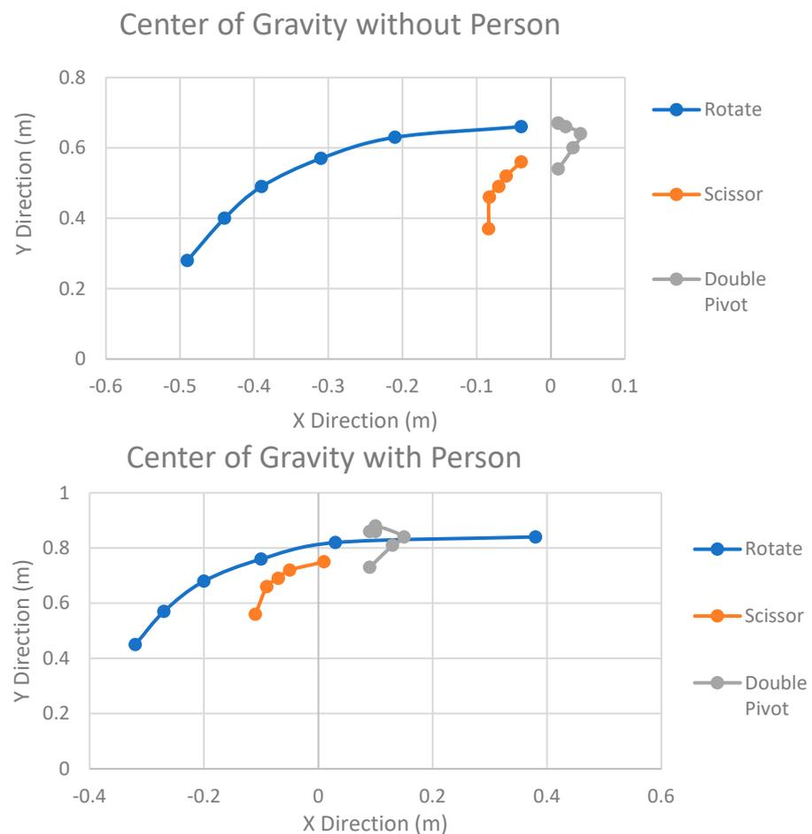
**Figure 8.** Center of gravity with and without a patient: rotate (Design 1), scissor (Design 2), double pivot (Design 3).
