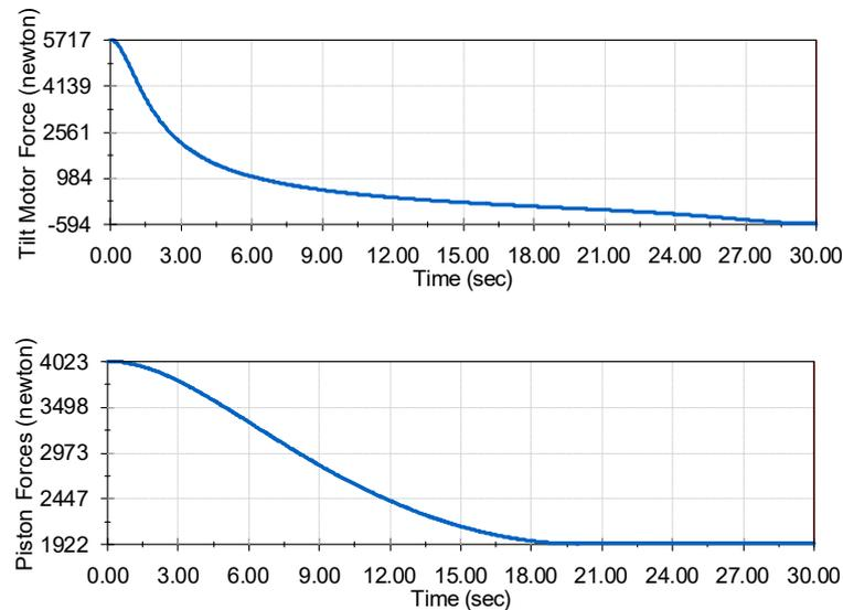
**Figure 11.** Design 2 (scissor lift) force results. Top: forces imposed on the linear actuator during movement from 0 to 90 degrees. Bottom: forces required by the piston to move from 0 to 90 degrees.
