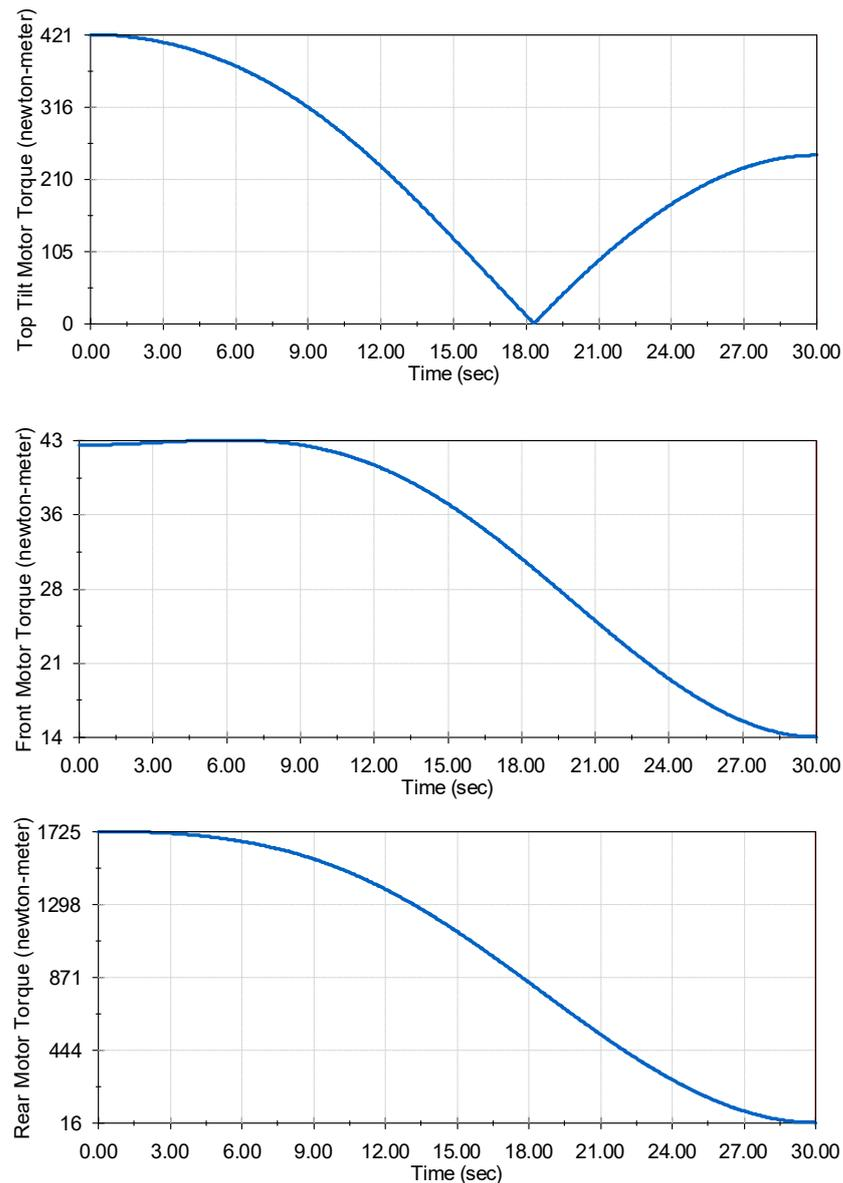
**Figure 10.** Design 1 (rotational lift) torque results. **(Top):** torque on the top motor when moving from 0 to 90 degrees. **(Middle):** combined torque on the two front lower motors that control the lift. **(Bottom):** combined torque on the two back motors which control the lift mechanism.
