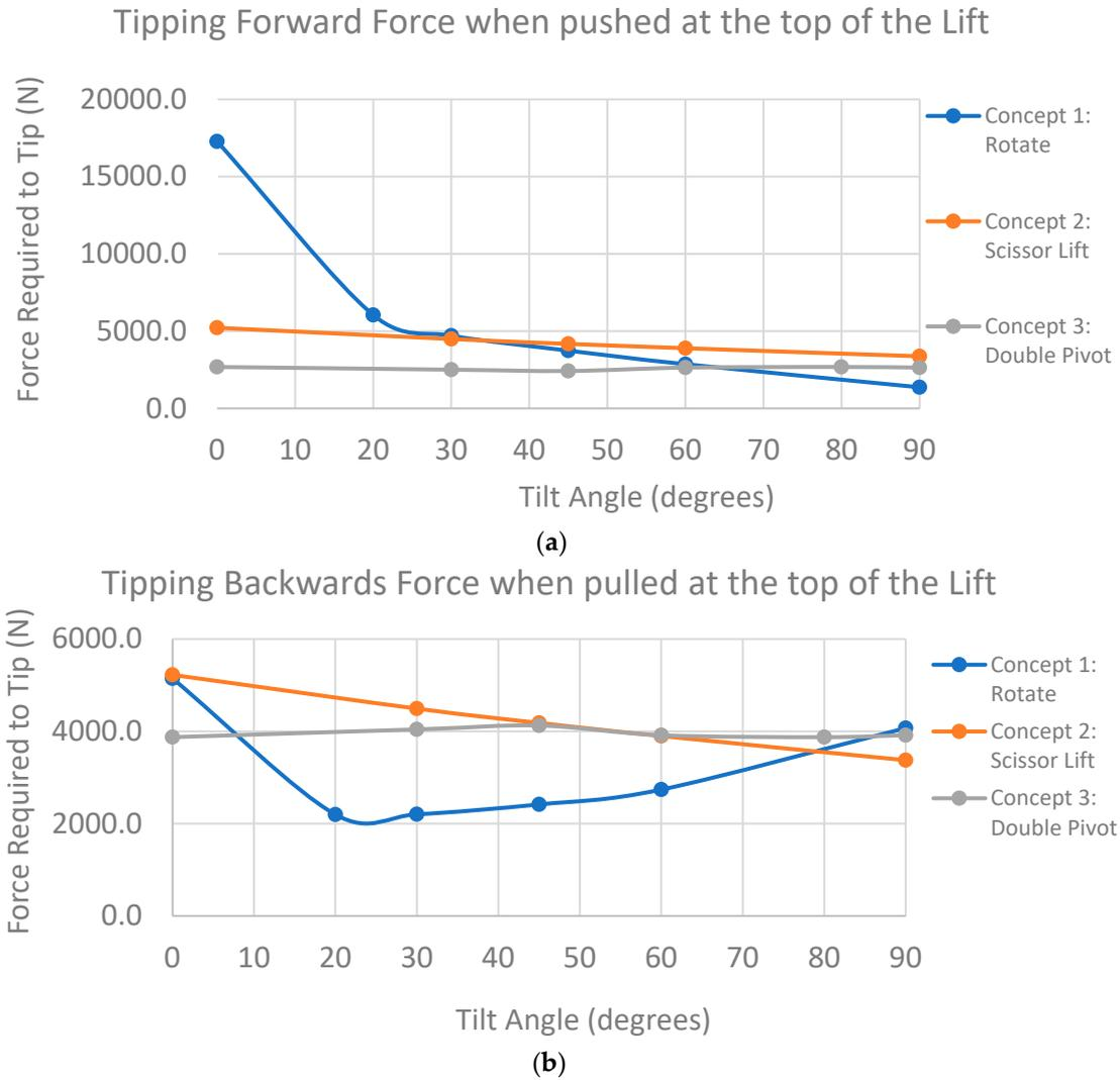
**Figure 9.** Tipping forces: (a) tipping forward results and (b) tipping backward results.
