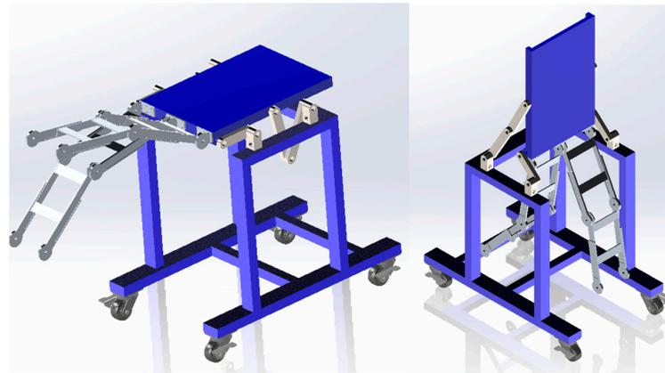
Figure 6. Concept 3—double pivot lift CAD model.
