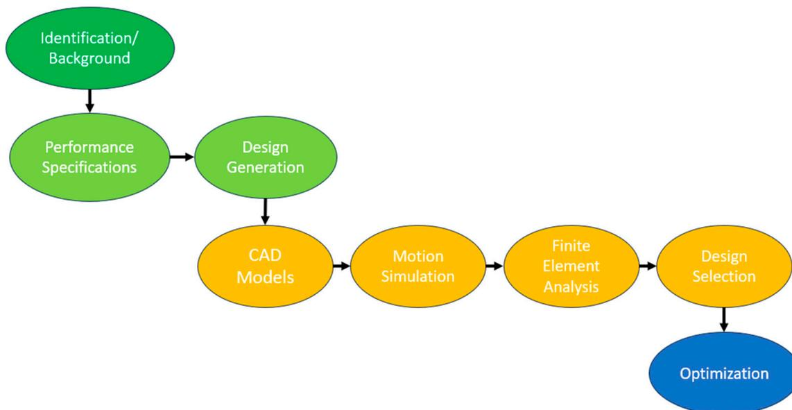
**Figure 1.** Design process/workflow steps.
