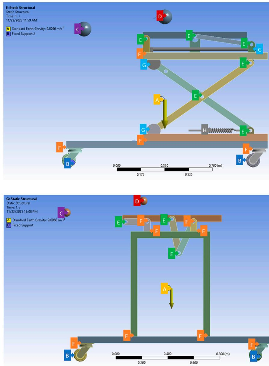
**Figure 2.** FEA constraints. Top: constraints for Concept 1—rotational lift; middle: constraints for Concept 2—scissor lift; bottom: constraints for Concept 3—double pivot lift. FEA constraint letters and colorization are listed below:
