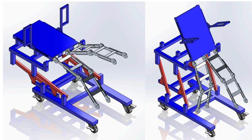
**Figure 4.** Concept 1—rotational lift CAD model.
