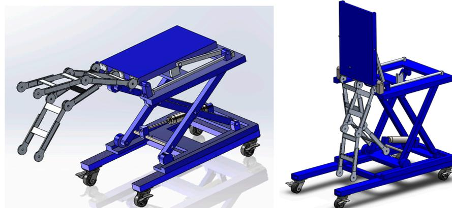
**Figure 5.** Concept 2—scissor lift CAD model.
