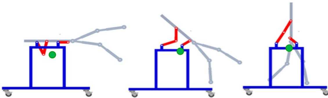
**Figure 7.** Center of gravity analysis; the green circle represents the center of gravity (CoG) of the RWTD.
