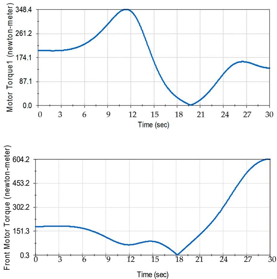
**Figure 12.** Design 3 (double pivot lift) torque results. Top: torque on the back motor which controls the larger pivot. Bottom: torque on the front motor which controls the smaller pivot.
