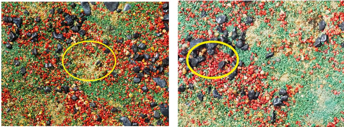
**Figure 11.** Sheet erosion occurs after erosion of G4.
