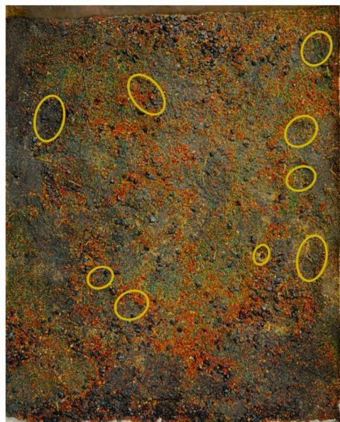
**Figure 14.** Pits after Erosion of G5.
