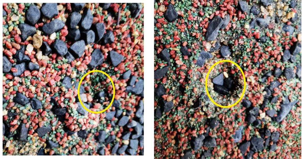
**Figure 8.** Pits occur after erosion of G2.
