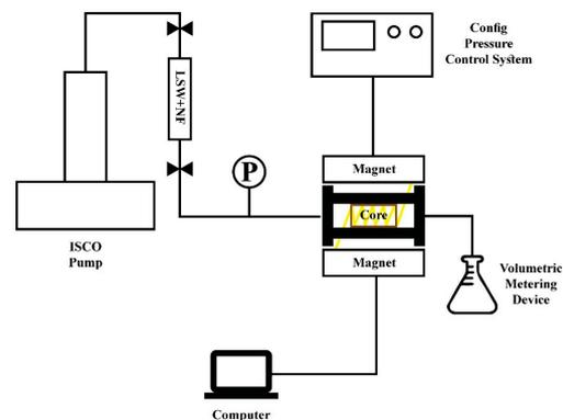
**Figure 4.** Schematic diagram of NMR experimental setup.
