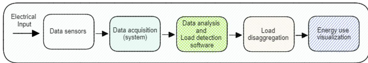
**Figure 1.** Steps of Intrusive Load Monitoring (ILM).
