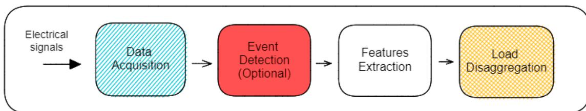
Figure 5. Steps of Non-Intrusive Load Monitoring (NILM).
