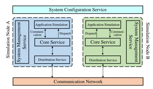
Figure 2. DIS simulation system architecture.
