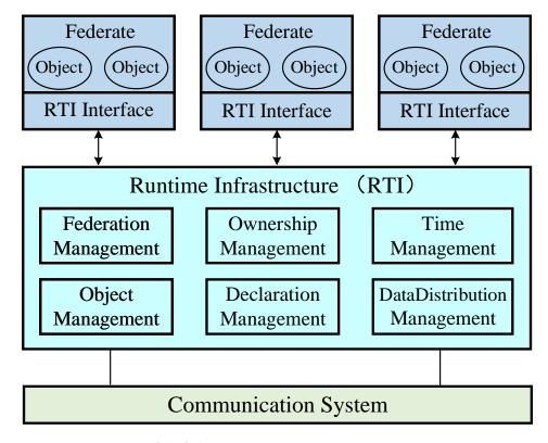
Figure 3. Construction of the federation in an HLA.
