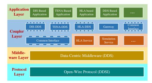
Figure 4. LSA simulation system architecture.
