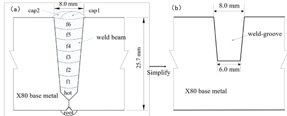
**Figure 2.** Schematic diagram of the simplified groove: (a) double V-shaped groove during actual welding process; (b) Simplified groove in the experiment.
