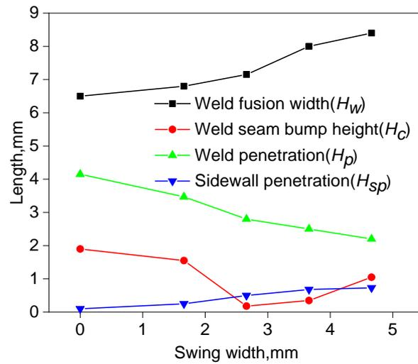
Figure 6. Effect of the oscillation width on the weld cross-section.
