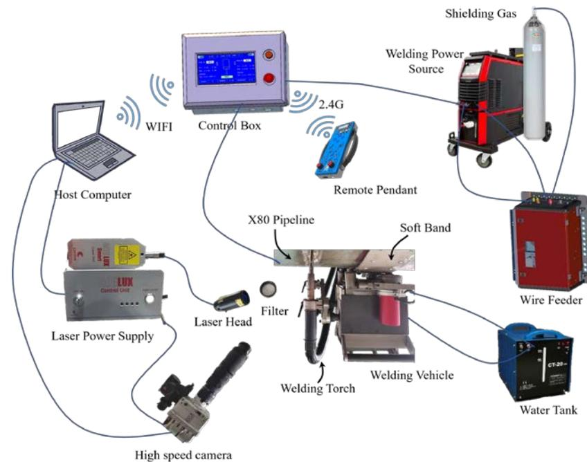
**Figure 1.** Schematic diagram of the oscillating arc NG-GMAW overhead welding.
