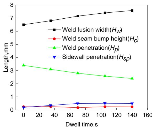
Figure 7. Effect of the sidewall dwell time on the weld cross-section.
