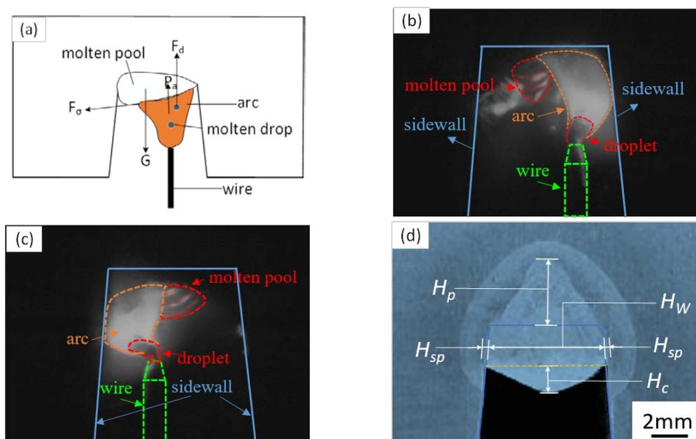
**Figure 4.** Weld formation of NG-GMAW overhead welding: (a) Forces acting on the molten pool. (b) High-speed camera image of the arc on the right sidewall. (c) High-speed camera image of the arc on the left sidewall. (d) Weld section morphology.
