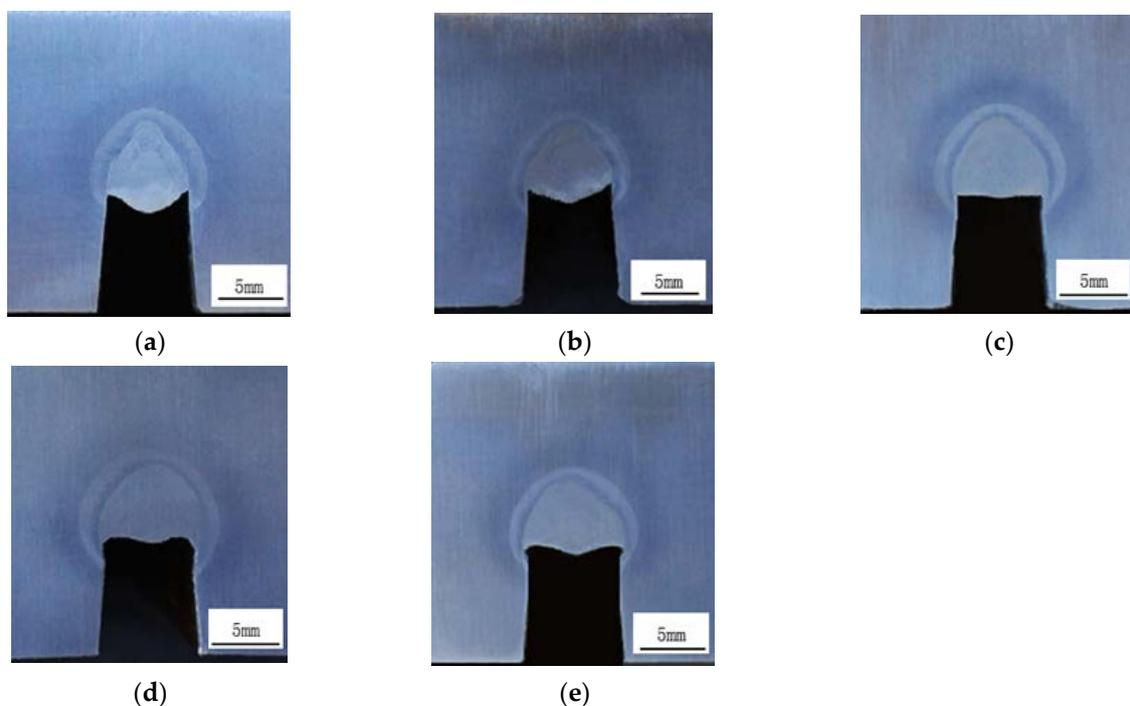
**Figure 5.** Weld cross-sections with different oscillation widths: (a) 0 mm; (b) 1.66 mm; (c) 2.66 mm; (d) 3.66 mm; and (e) 4.66 mm.
