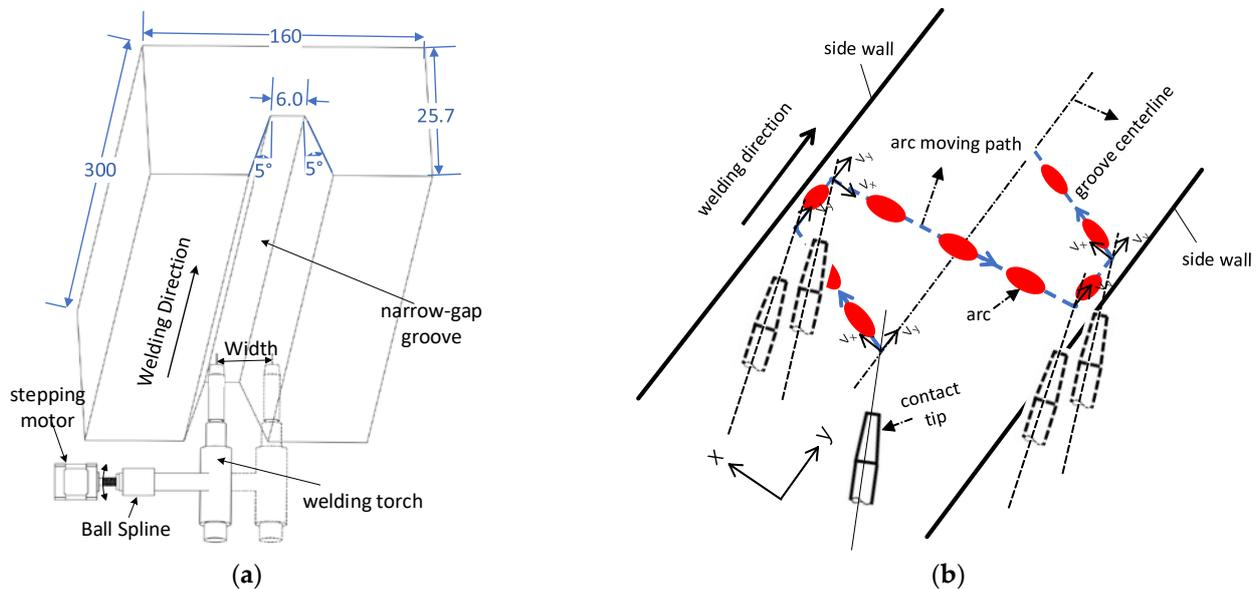
**Figure 3.** Schematic diagram of: (a) straight oscillating arc mode; and (b) oscillating arc welding track.
