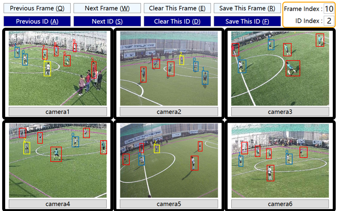
Figure 4. GUI of our self-designed multi-camera annotation software. The software allows annotators to quickly assign corresponding identities and adjust the size of detection predictions in auxiliary cameras by connecting them to bounding boxes in camera-1. (1) The bounding boxes in camera-1 are based on manual annotations, whereas the bounding boxes in other cameras are generated by the detector. (2) The purple lines serve to demarcate the target area [9]. (3) The blue bounding box has been adjusted to the correct size and aligned with the identities across multiple views. (4) The yellow bounding boxes are being adjusted and aligned. (5) The red bounding boxes are waiting to be adjusted and aligned. (6) The number above the bounding box indicates its identity. (7) The software utilizes calibration parameters to approximately locate the detection predictions in auxiliary camera views.
