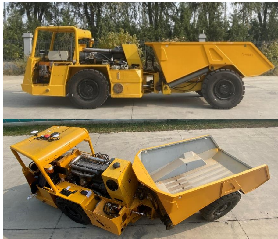
Figure 7. Articulated dump truck configuration.
