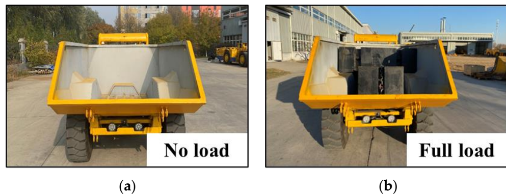
Figure 6. Articulated dump truck with no-load condition and full-load condition: (a) no load; (b) full load.
