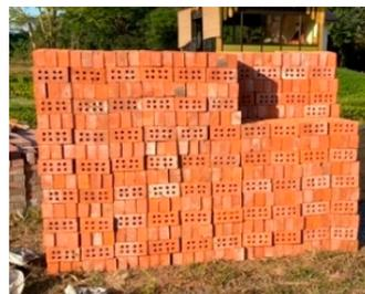
**Figure 3.** Perforated brick.
